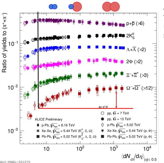
ALICE has measured the ratio of strange to non-strange hadron yields versus multiplicities in different collision systems and energies
