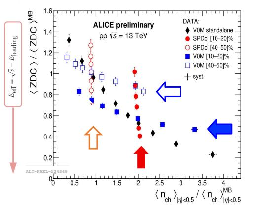
A multi-differential analysis in combined V0M and SPD classes allows to disentangle the effective energy and the multiplicity at midrapidity Standalone V0 event classes
