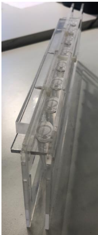
Eppendorf and films holder for multiple irradiations in a water tank
