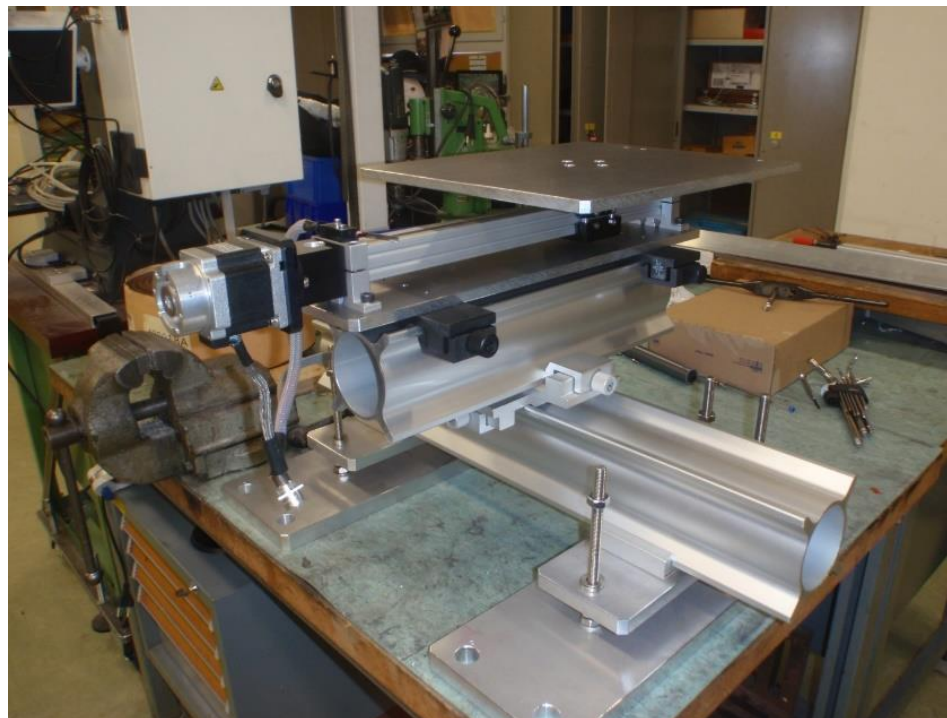
Motorized table for water phantom displacement
