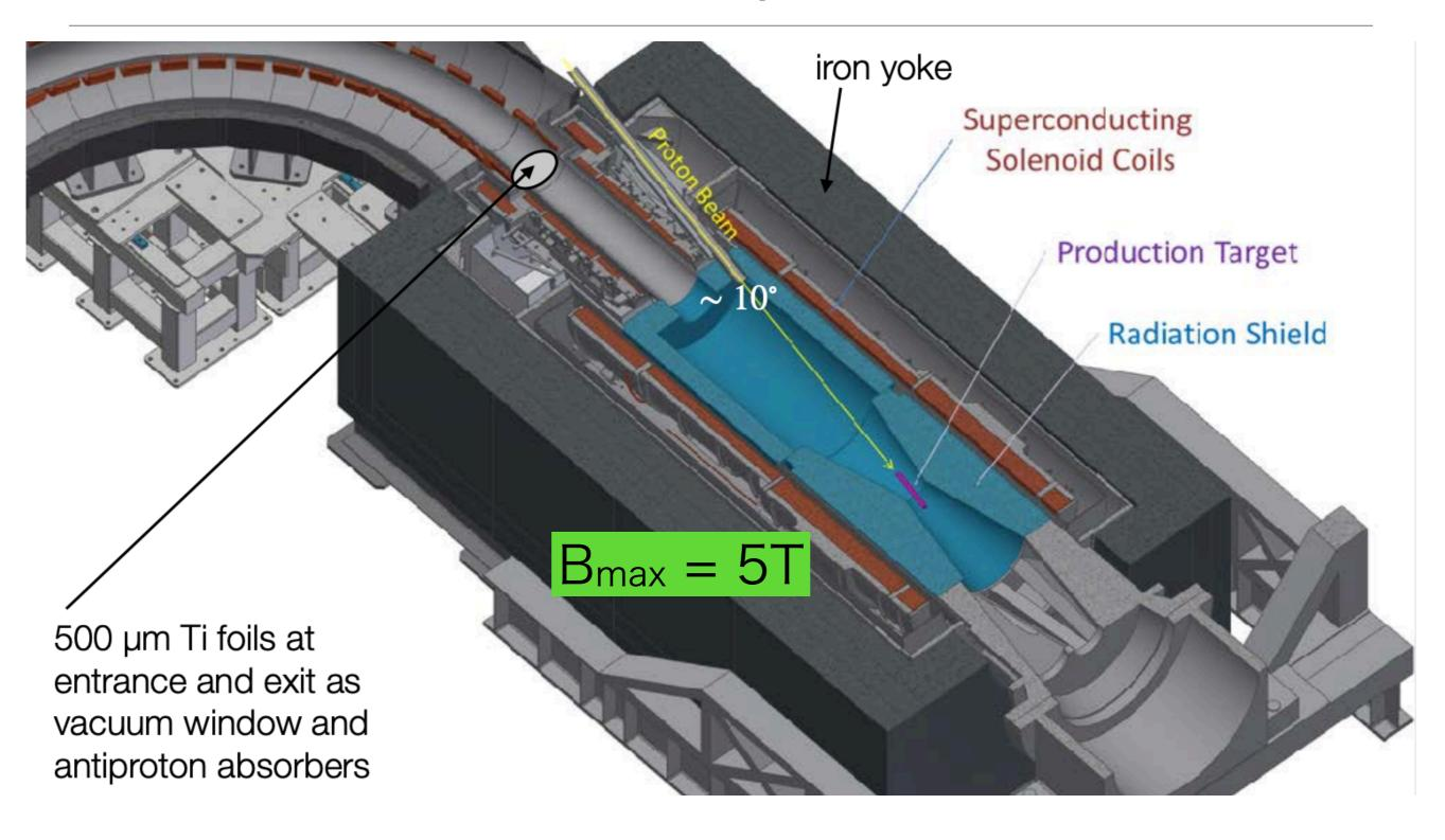
Superconducting solenoid magnet
