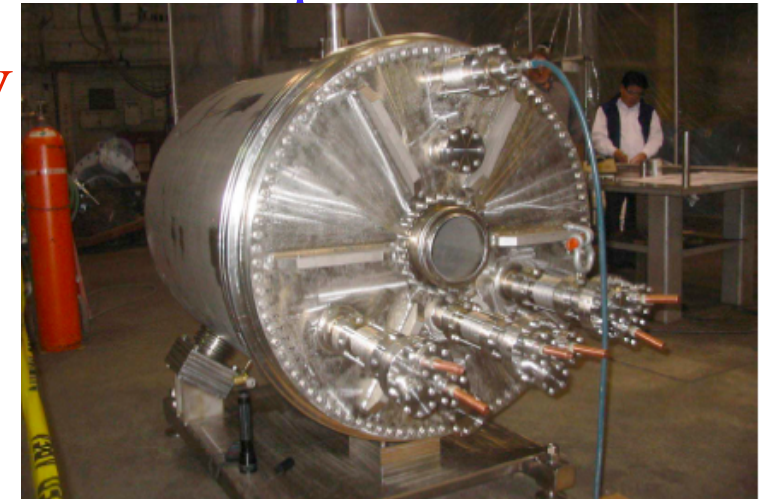
15-T NC pulsed solenoid:
