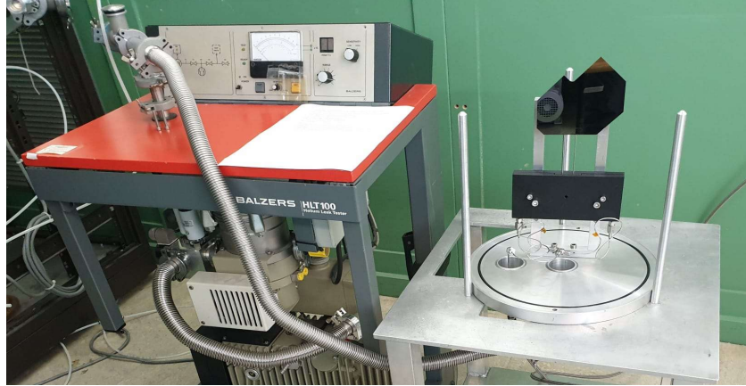
High pressure helium leak test (60 bar)
