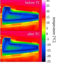
No degradation of thermal performance of cores is observed after thermal cycling.
