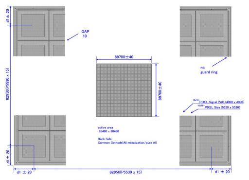
d1 : Center of corner PIXEL to chip edge : 3375
