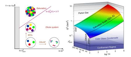
Dependence of saturation on rapidity, transversal impulse and atomic number of the target
