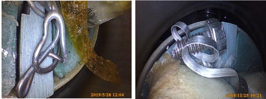
Metallic debris found in diode boxes
