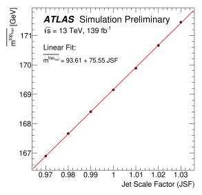
Calibration line obtained by shifting JSF and register the effect on jet mass  $JSF = 1.00035 \pm 0.00087$
