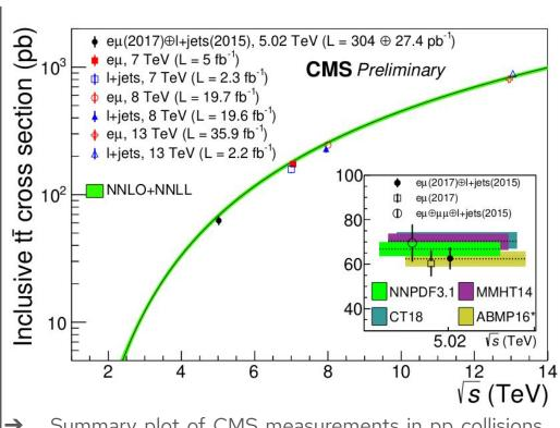
Summary plot of CMS measurements in pp collisions at different center-of-mass energies.
