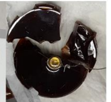
CTD 101K After 10 Thermal Cycles
