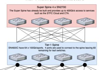
A protocol known as Equal Cost Multi Pathing (ECMP) is used to ensure traffic uses all the spine links.
