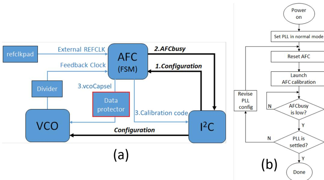
Figure 2: Block Diagram of AFC (a) and its fully automatic calibration workflow (b).
