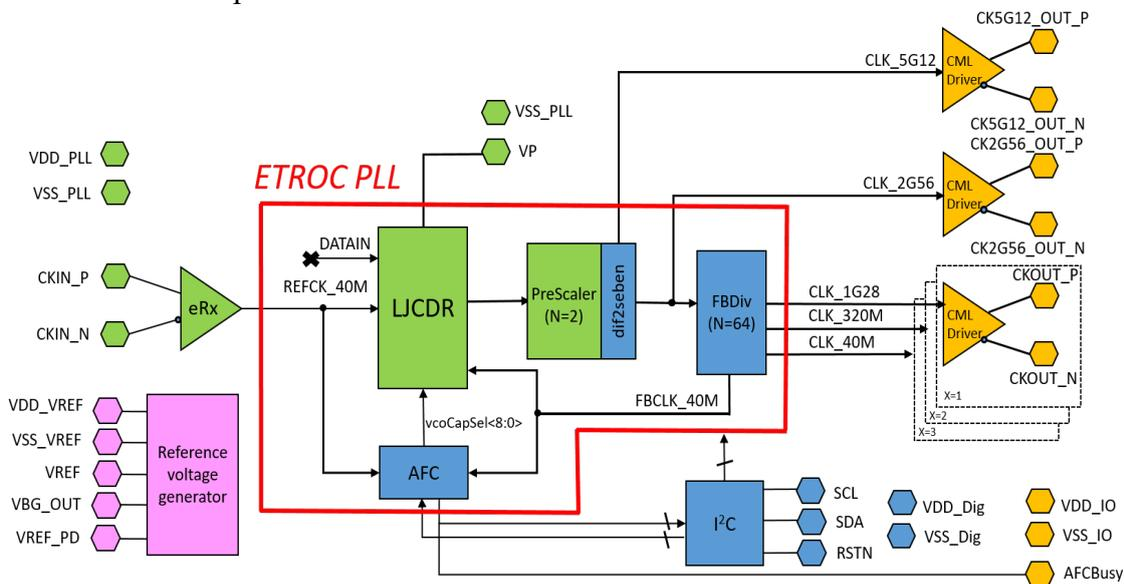
Figure 1: Block Diagram of ETROC PLL
