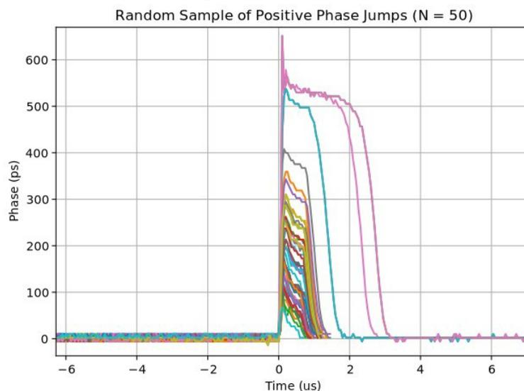
Figure 5: Random sample of positive phase jumps during heavy ion irradiations.
