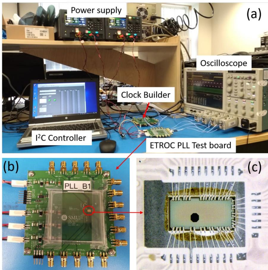
Figure 3: Lab test setup (a), test board (b), and wire-bonded chip (c) of ETROC PLL.
