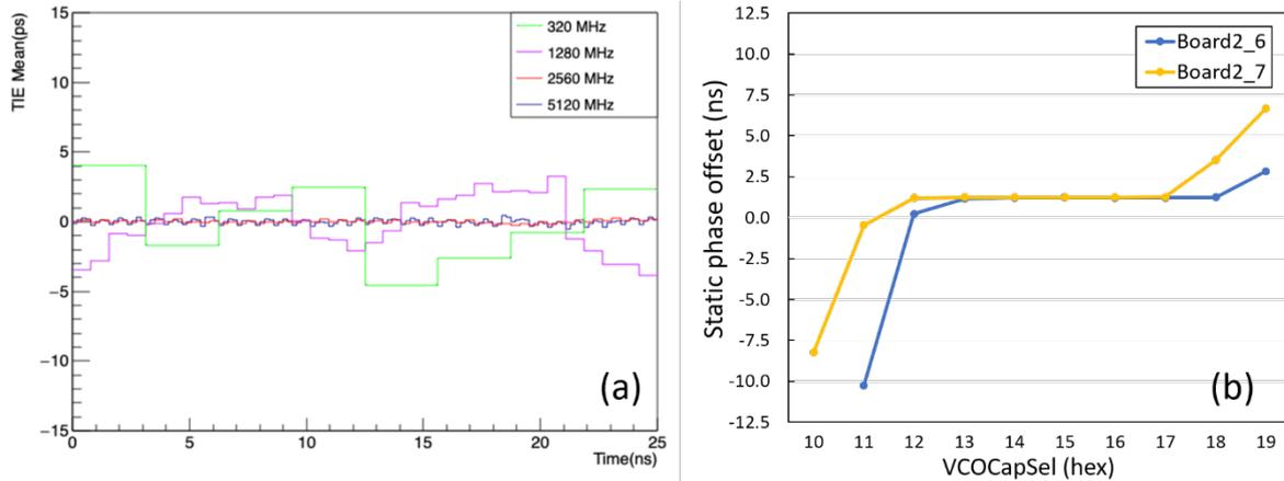
Figure 4: TIE jitter of output clocks with different frequencies (a) and static phase offset versus VCO capacitor bank setting (b).
