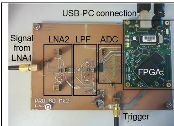
Figure 1 – Detector electronics board
