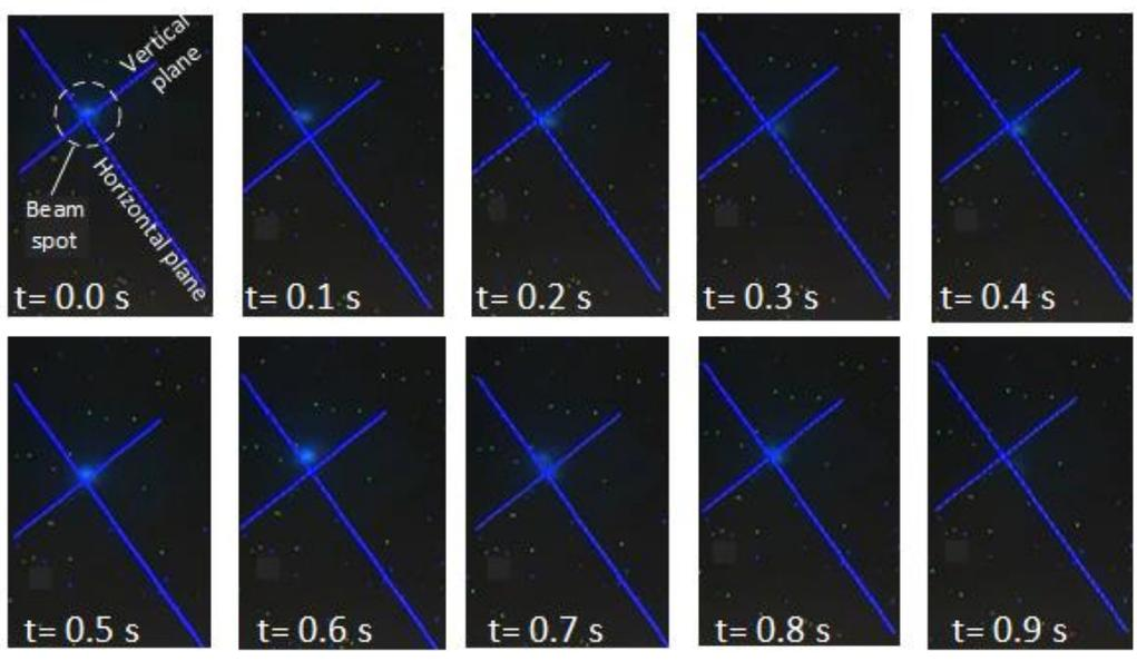
Figure 5 – Slow beam oscillations around the horizontal axis are observable by measuring the ionoacoustic signal amplitude over time
