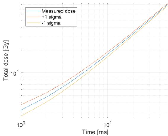
Figure 3 – Measured cumulative dose vs. time with +/- 1-sigma precision
