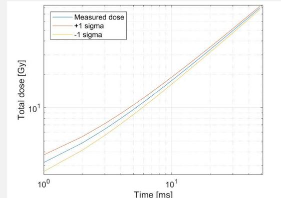
By characterizing the noise performances (62.9 mVRMS, equivalent to 363 mGyRMS, from sensor and electronics thermal/flicker noise) it is possible to measure the dose deposition variations due to random beam fluctuations over time, equal to 138 mGyRMS or 8.6% of proton number/shot. The cumulative dose after 50 shots (50 ms acquisition) is 77.56 Gy  $\pm$  2.75 GyRMS (3.43%).
