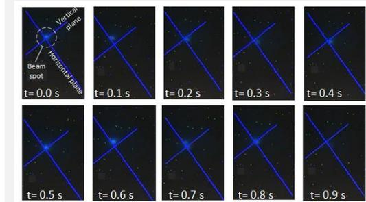
Finally, the ionoacoustic signal amplitude has been recorded for 1 s. By low-pass filtering, a slow  $\sim 7$  Hz fluctuation in the ionoacoustic signal amplitude becomes observable. Such slow fluctuation is compatible with the beam fluctuation around the horizontal beam axis visible in the CCD beam spot monitoring system.
