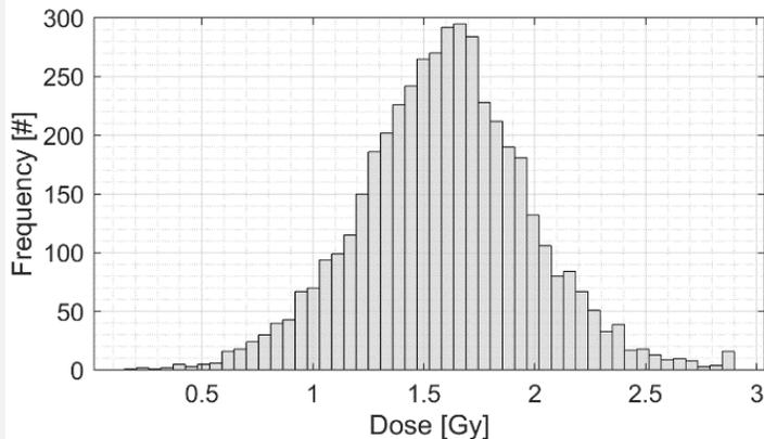
Measured acoustic sensor output signal is 276 mV0-peak corresponding to 1.59 Gy dose at the Bragg peak, consistent with 1.6 Gy dose/shot calculated from the beam current and Bragg peak physical size. By repeating the measurement 8000 times, the measured dose precision has been found equal to 388 mGyRMS (24.4%) due to random noise fluctuations.
