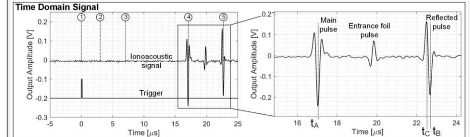
The ionoacoustic signal from 20 MeV protons has 2 MHz frequency and is characterized by a main pulse and a reflected pulse. The amplitude of the main pulse is proportional to the dose deposition at the Bragg Peak and can be used to measure the beam current.
