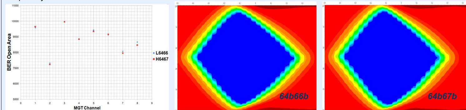
Figure 4. Left: BER Open Area comparison of 64b/66b (blue) and 64b/67b (red). Right: Eyescan of a link running the 64b66b version of the protocol (left) and one of the same link running the 64b67b version of the protocol (right).
