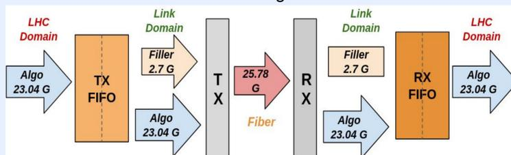
Figure 2. Asynchronous architecture block diagram. In the case of 25 G links, the actual line rate 25.78125 Gbps. The maximum Algorithm clock can run at 360 MHz, resulting in bandwidth of 23.04 Gbps. The remaining 2.74125 Gbps occupy the so called Filler Bandwidth which on the must be identified on the receiving end and not be written on the RX FIFO block.
