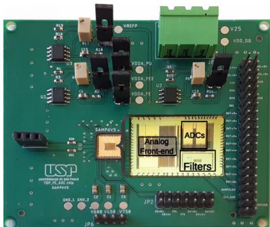
Figure 2: Test board with the open package and a zoomed version of the die showing its internal blocks.
