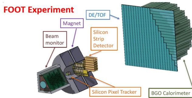
CAD representation of the FOOT experiment configuration with all the detector sub-systems. The beam goes from the bottom-left corner to the top-right one.
