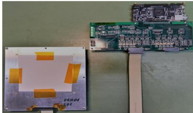
MSD data acquisition system (a single plane micro strip detector inside the metal box, hosted on the printed circuit board, the printed board hosting the ADCs and the DE10 nano board). The picture misses one hybrid board for the MSD layer to be complete.
