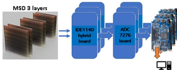
Block diagram of the MSD showing three replicas of detector layers. For each layer, from left to right, the 2-plane detector, the IDE1140 readout, the ADC board, and a DE10-Nano. The arrows show the direction of the data flow.
