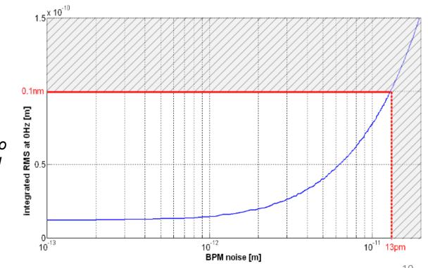
Sensor's noise has to be < 13 pm integrated RMS @ 0.1 Hz
