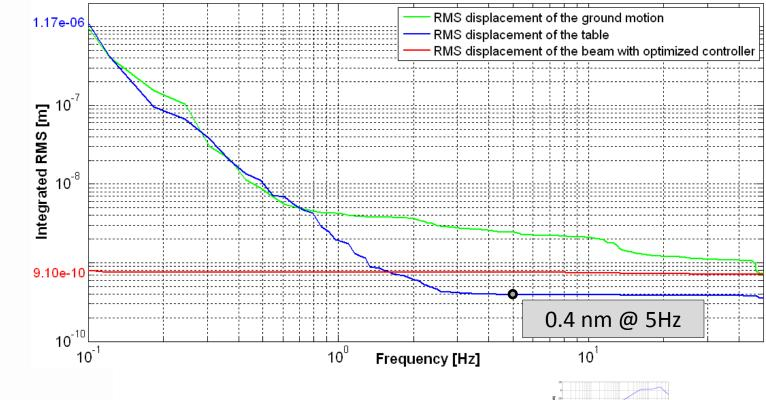
• Efficiency of the feedback scheme: 0 Hz to 2 Hz
