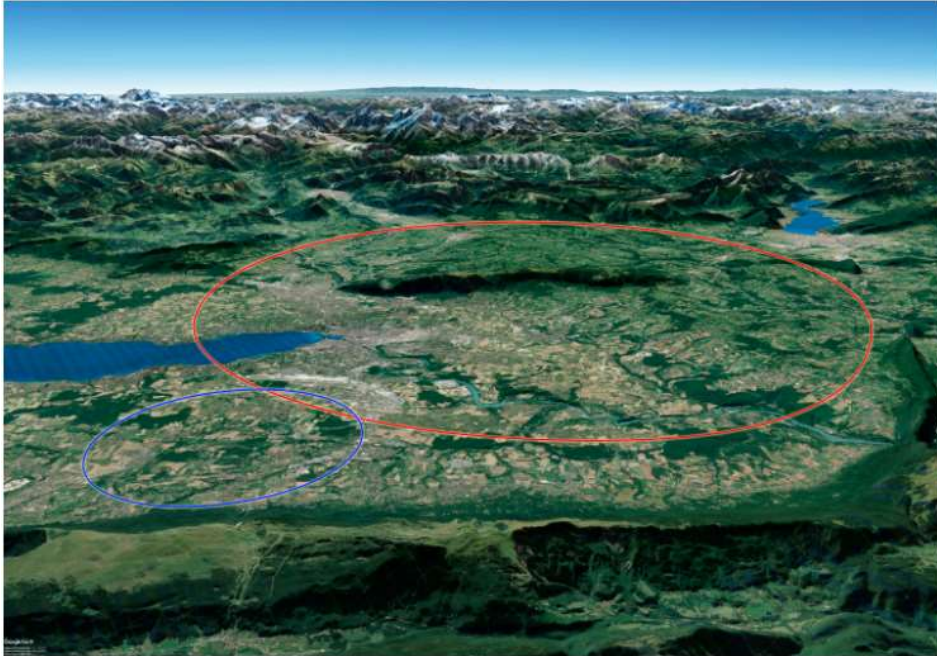
The FCC study prepared a conceptual design of a 100km long ring accelerator, that uses CERN's existing accelerator infrastructure. (Image: CERN)
