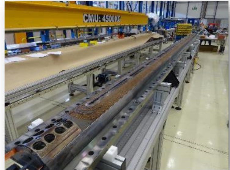
MQXF & FRESCA Magnet Impregnation & Curing Tools
