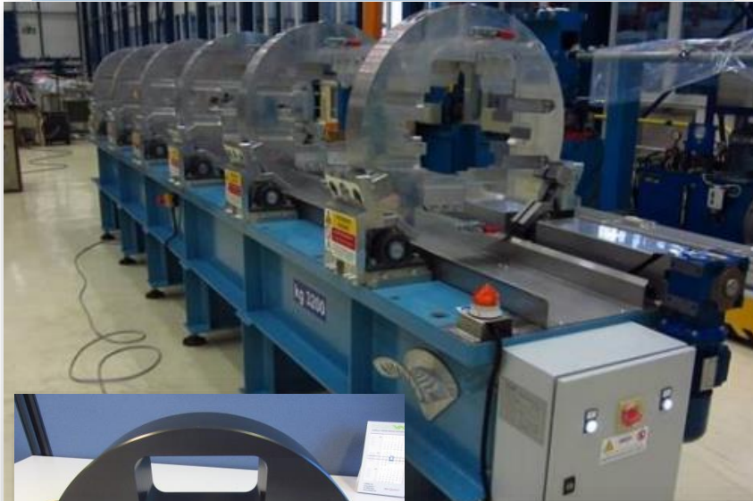
Rotating Table for SC magnets assembly
