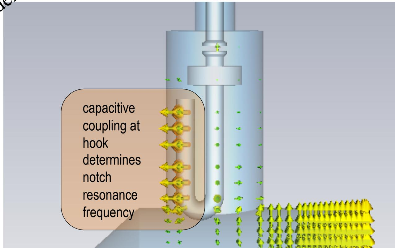
strong capacitive coupling between "hook" and outer conductor
