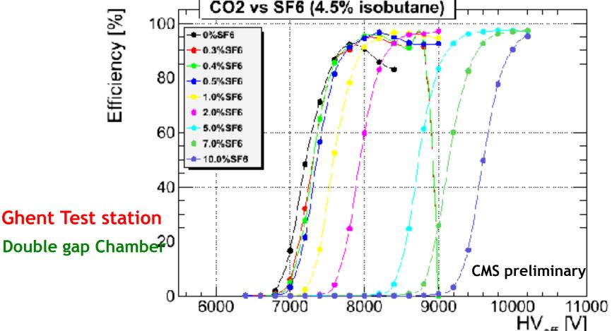
HV<sub>eff</sub> [V] For high values of the applied voltage one of the Gaps trips and the chamber works in single mode.
