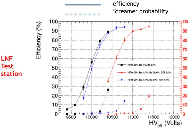
HV normalized to P=990 mbar and T= 20 oc
