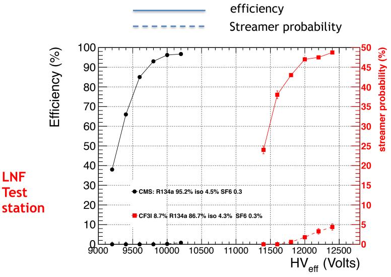
HV normalized to P=990 mbar and T= 20 oc
