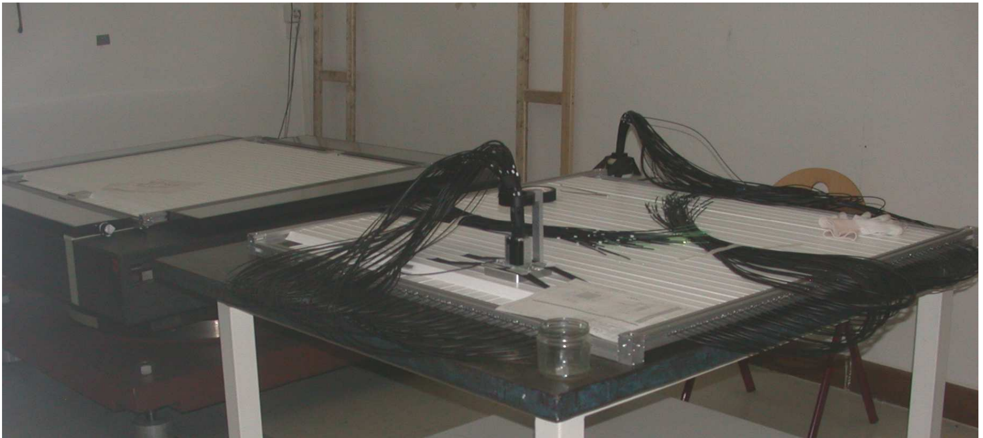
Above, the assembly stands of EMR planes(1 for plane assembly, 1 for module assembly)
