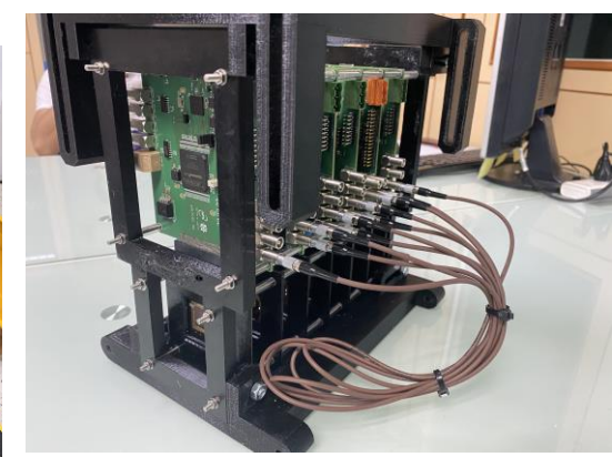
ALPIDE holder with Aluminium support
