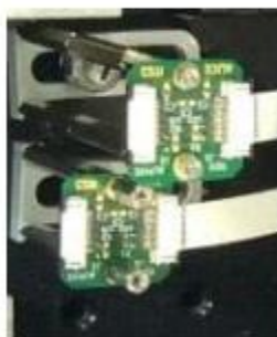
I-board (FPC to long flex; lessens tension)
