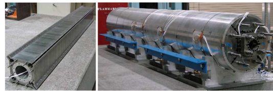
Fig. 4. LQSD dummy coil-pack and final assembly after pre-load.
