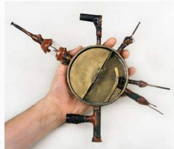
Livingstone cyclotron, diam. 10 cm. 80 keV protons
