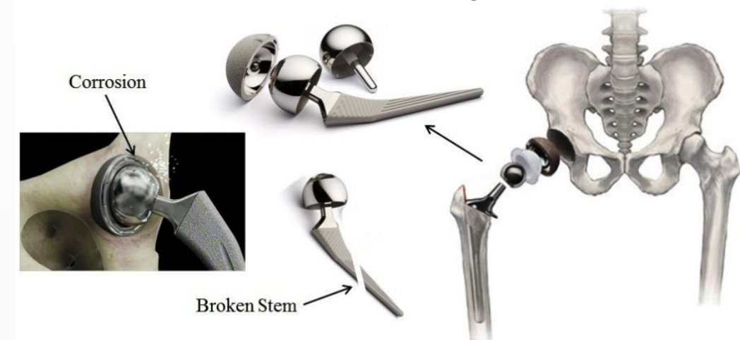
Corrosion for implanted 304 SS (A. Nikmah et al 2019 IOP Conf. Ser.: Mater. Sci. Eng. 515 012018)
