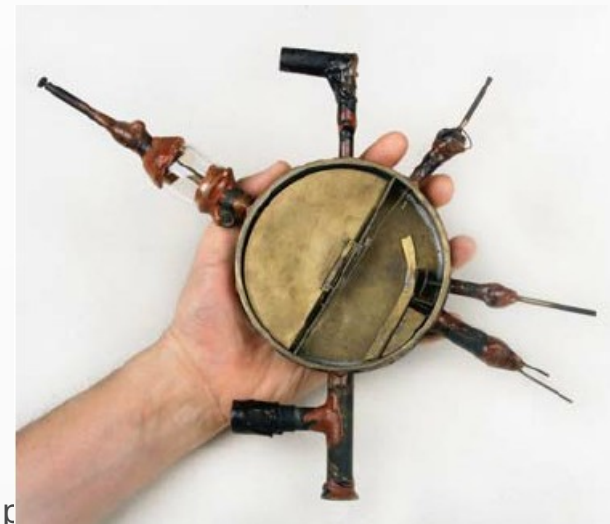
Livingstone cyclotron, diam. 10 cm. 80 keV protons
