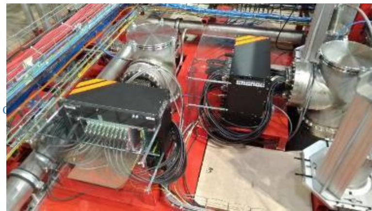
Top drift electronics from Dual-Phase design
