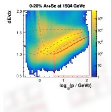
Selection of protons is based on dE/dx measurements in TPCs:
