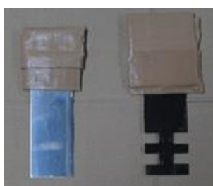
Fig.2 Two types of stirring plates
