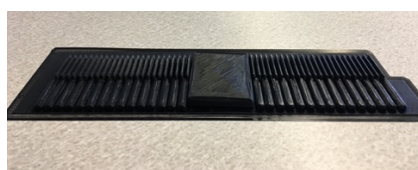
Fig. 1 A ridged surface to measure the speed of a ball
