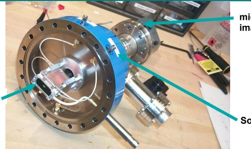
microchannel plates and imaging CCD
