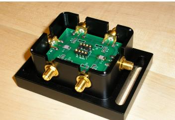
Photoconductive GaAs switch for triggering
