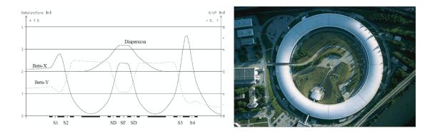
The DBA structure provides a lower natural emittance than a FODO lattice with the same number of dipoles.
