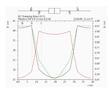
Outside the dipole, the emittance is relatively large. This is not ideal for a light source, since insertion devices at locations with large dispersion will blow up the emittance.
