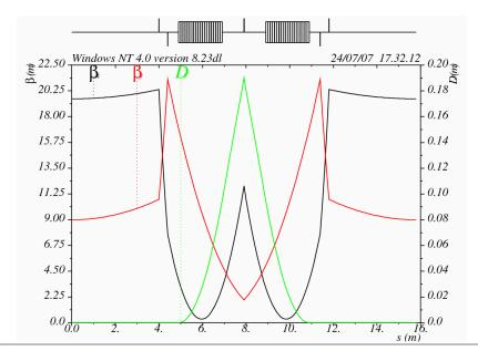
To calculate the natural emittance in a DBA, let us begin by considering the constraints needed to achieve zero dispersion at either end of the cell.
