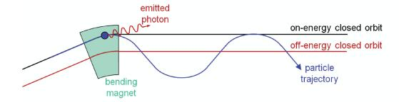
The beam eventually reaches an equilibrium distribution determined by a balance between the radiation damping and the quantum excitation.
