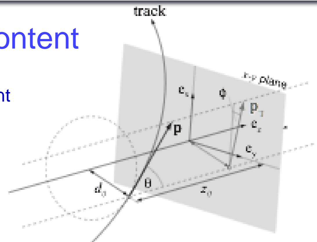
These are the track parameters which define the kinematics of this *TrackParticle*.
