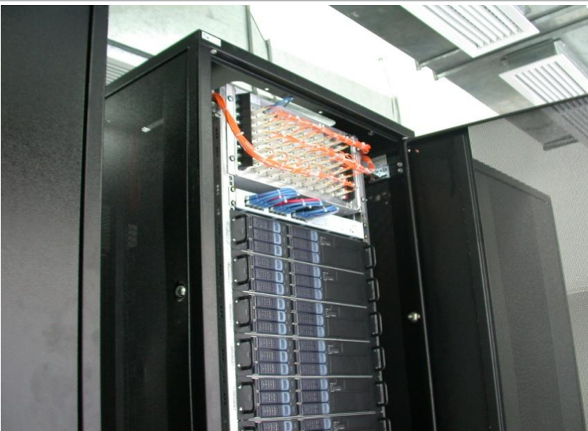
Cluster configuration 64 nodes with two Xeon 3GHz processors
