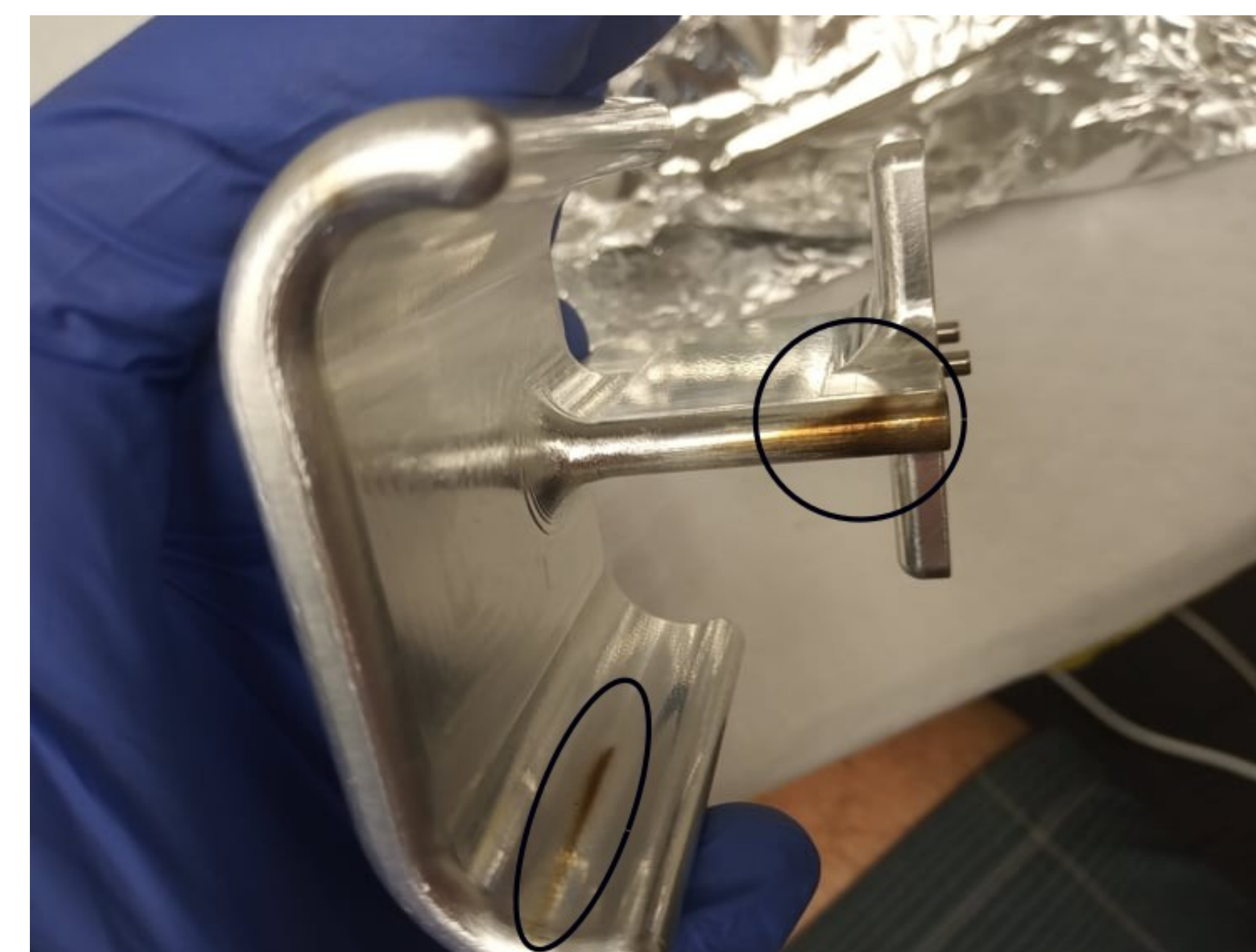
Figure 3: Wing electrode with scorch marks where electrons are dumped.
