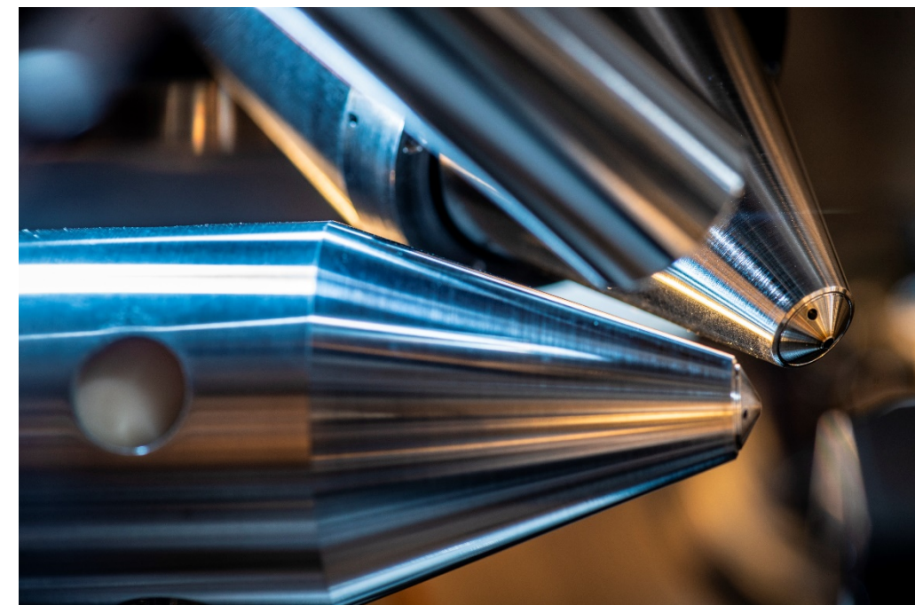
Objective lenses of the FIB, FEB and tip of the SED.
