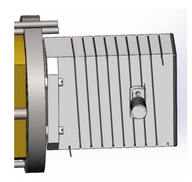
Layout of the internal oven. the diameter of the internal oven is 10 mm, and the sample capacity is designed as 20 g.
