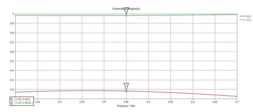
The microwave transmission and S parameters of the matching waveguide is simulated by CST.
