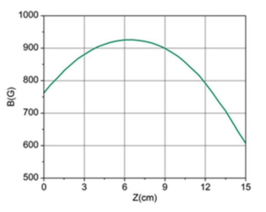
The axial magnetic field distribution along the plasma chamber.
