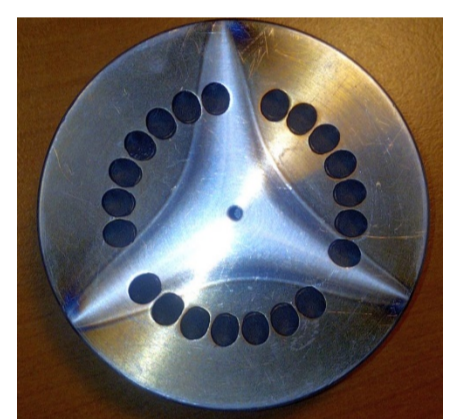
Erosion on the plasma electrode shows plasma symmetry
