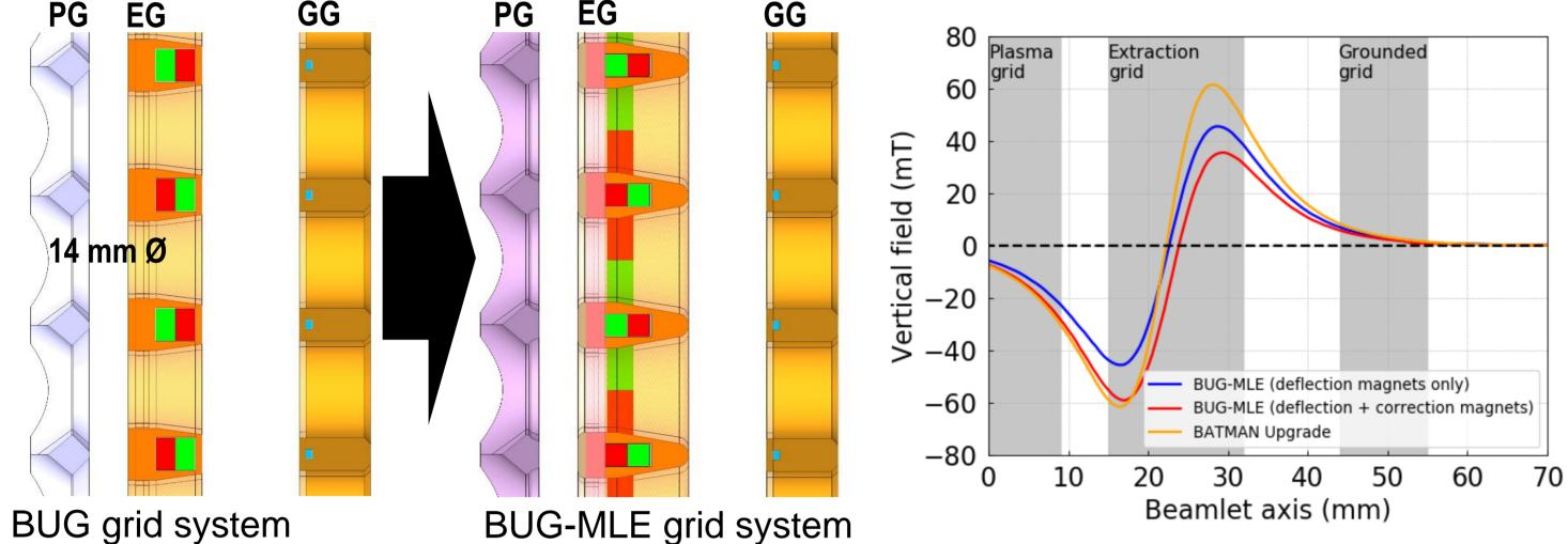
Deflection correction magnets add horizontal component to magnetic field Horizontal component focuses/defocuses vertically: increased divergence!
