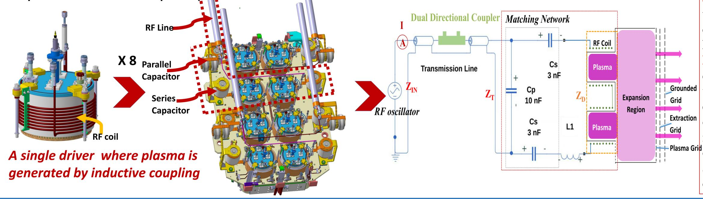
Aim 2): Explore driver impedance variation in various experimental conditions, like RF power, gas pressure, PG current, type of gas, Cesium, etc. **Motivation:** driver impedance is mutually coupled to the plasma which has a variable impedance depending on the experimental conditions. The knowledge of variation in driver equivalent impedance can lead to an accurate design of matching network which can allow to achieve transfer of full power to the driver.
