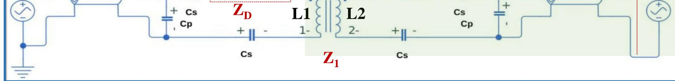
Analytically, the impact of mutually coupling on driver impedance  $Z_D$  is found to be negligible (< 5) %) assuming 5  $\Omega$  and 20  $\mu$ H for drivers resistance and inductance with plasma. Therefore, only a single RF circuit has been considered!
