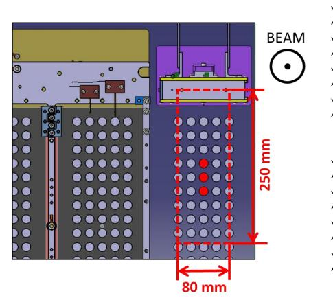
$\blacktriangleright$  Placed at 600 mm from the grounded grid [4] Centered on a top beamlet group
