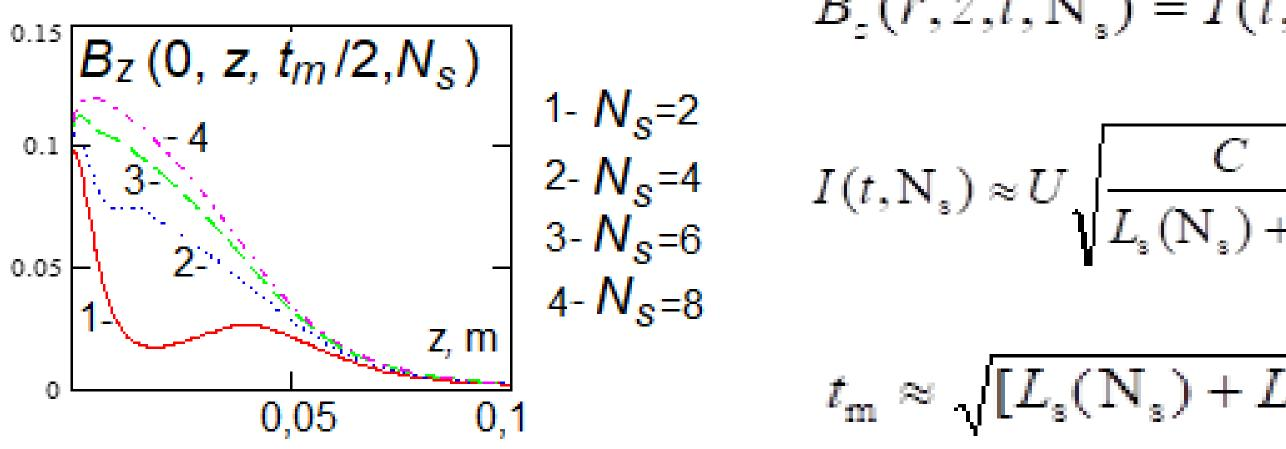
The calculation showed that the optimal option is Ns = 6. The expansion of the laser plasma in an external HSMF leads to an additional collective acceleration of its components. The use of CMF increases the pulse duration to 4.8 ms, and the number of particles from  $3 \times 10^{11}$  to  $2,3x10^{12}$ .
