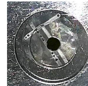
Traces from laser-alignment on the extraction side
