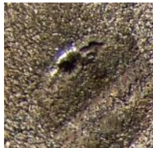
Laser-induced craters on the cathode surface during focusing attempts
