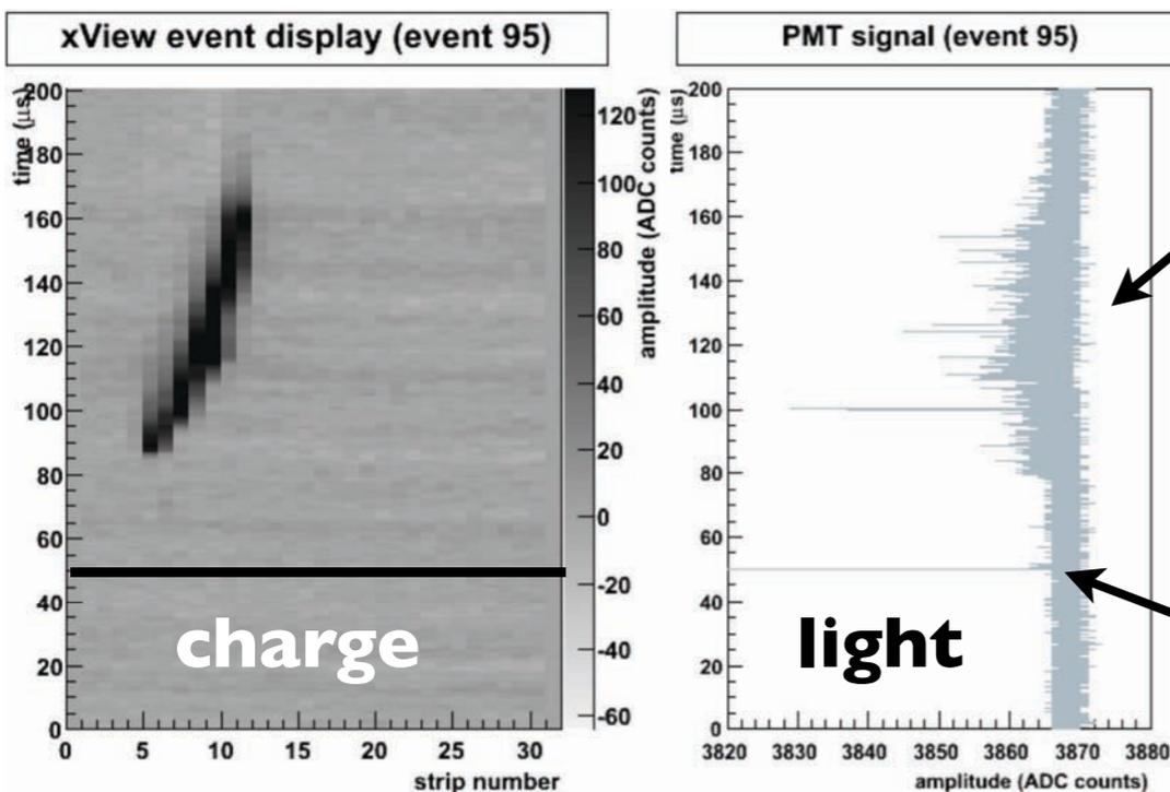
secondary scintillation light produced in GAr (field between extr. grids and micromegas)
