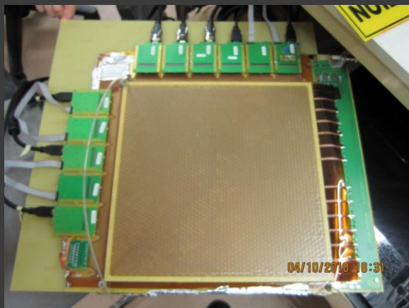
Triple GEM with 11 APV25 hybrids
